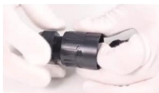
Unscrew the RJ45 plug bottom cover
