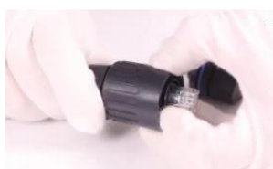
Tighten the waterproof connector
