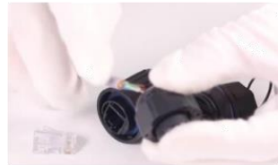
Insert the dialed network cable into the bottom cover
